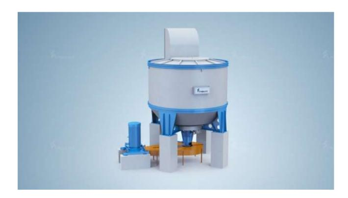
Yunda **ZDSZ Series middle consistency hydrapulper** is a kind of vertical pulp equipment, which is used for pulping various pulp boards, broke and waste paper, the pulping consistency is up to 5%-8%, as well as high defibering ability.
