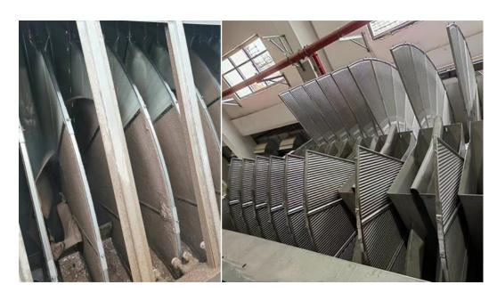
The machine is mainly composed of tank body, upper cover, main shaft, sector plate, web cleaner and drive device etc. The detailed structure is shown in the equipment general drawing.
