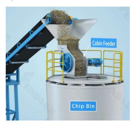
The cabin feeder consists of a bin body (1), an end cover (2), a transmission unit (3), an inspection and maintenance hole cover (4), a gear box (5), a transmission side bearing (6), and a driven side bearing unit (7), zero-speed switch bracket (8) and zero-speed switch (9) and other components.
